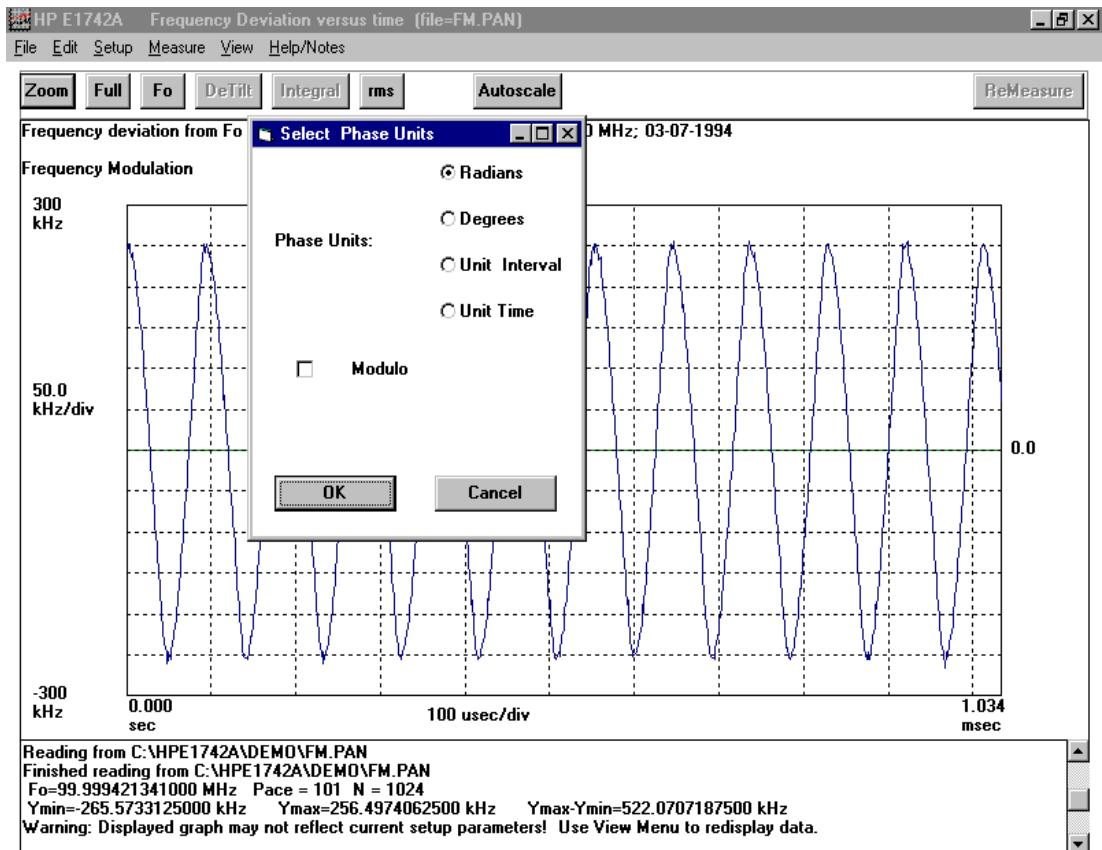
You can select units for the phase measurement results from this window. All phase displays will show the selected units on the Y axis. You can obtain other phase units by clicking on a point. The other units for that point will be shown in the Log display at the bottom of the screen.
