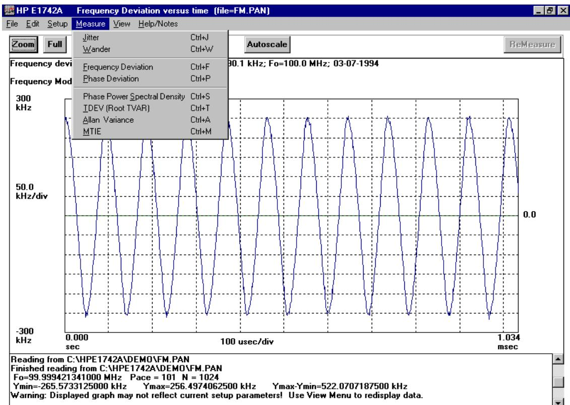
**MEASURE MENU VS VIEW MENU.** The choices on these two menus are very similar, however the action performed by the instrument is quite different. Selecting any of the choices on the **Measure** menu will cause the instrument to initiate a measurement and acquire a new set of data points and perform the selected result processing. Selecting any of the choices on the **View** menu will cause the instrument to perform the selected calculations *on the currently acquired data*.
