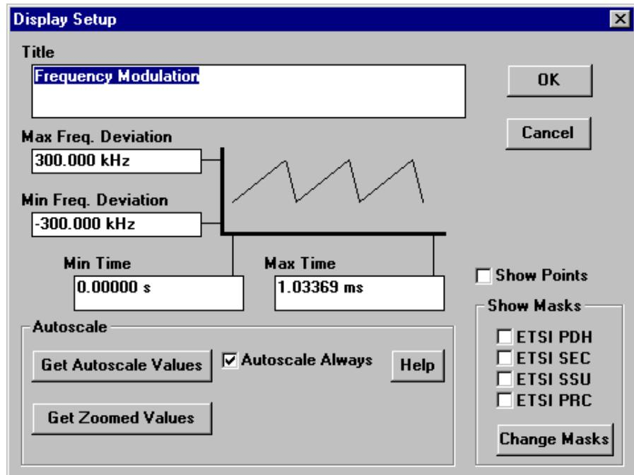
The Display Setup menu lets you annotate the display with a title, date, or other descriptive information which may be useful if you store the data to a file or print a hard copy. You can also set the scaling for both the x and y axis of the measurement display or select the **Autoscale** function. Display masks can also be turned on in the Display Setup dialog box. Search the HP E1742A/46A/48A on-line Help for **Show Masks** to obtain more information.
